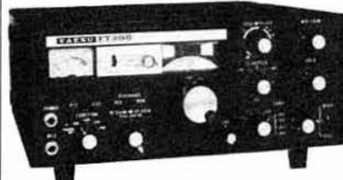
FT200B Transceiver 10-80m, 180W pip. Mains (FP200) or DC (DC200) PSU's.
