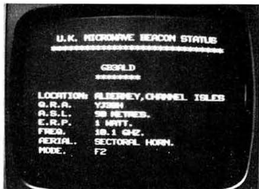
One of the pages of data currently being transmitted by the 10GHz beacon GB3LBH
