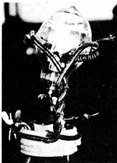
One of Fleming's early experimental diodes (Photo: Marconi Company)
