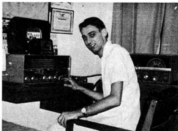
Adrian Sainsbury, VS9AAS, Khormaksar, Aden, 1964-1966. Equipment consisted of HT37 transmitter with SX111 receiver and quad at 90ft
